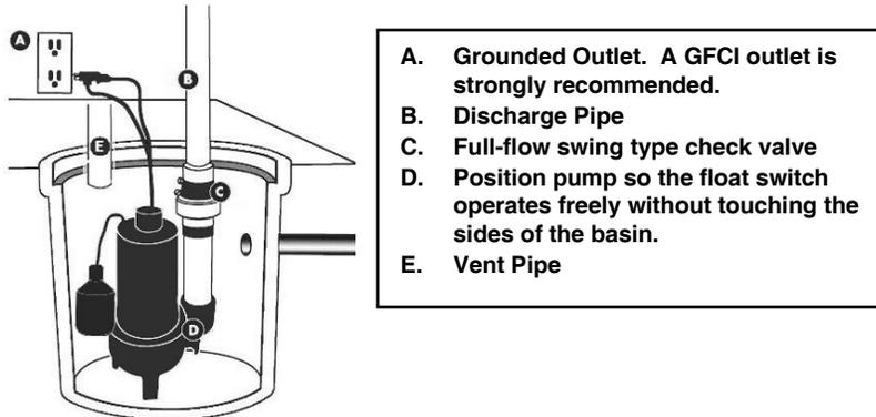
3. Install a full flow, swing type check valve (not included) as close to the discharge outlet on the pump as possible. A new check valve will greatly increase the life of your pump, and should be the same size as the pump discharge, in this case 2".
